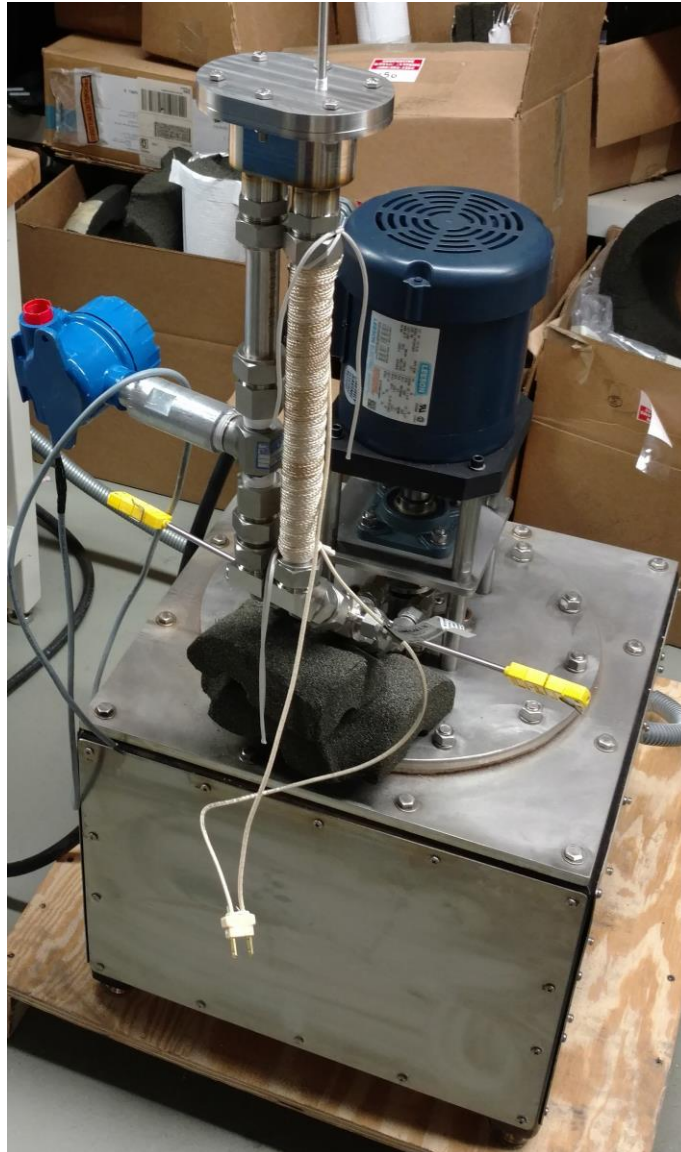
Figure 3-11 Pump and Melt Tank
