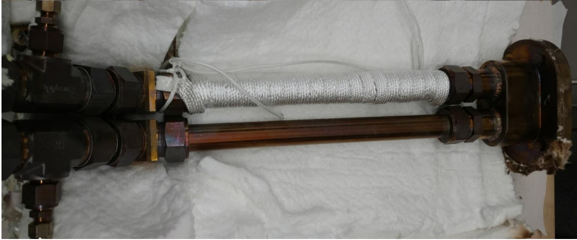
Figure 3-25 Post salt shakedown test loop
