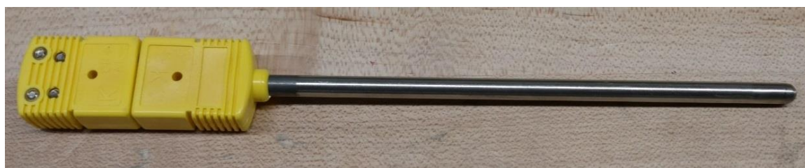
Figure 3-13 1/4" Diameter Omegaclad K-type thermocouple
