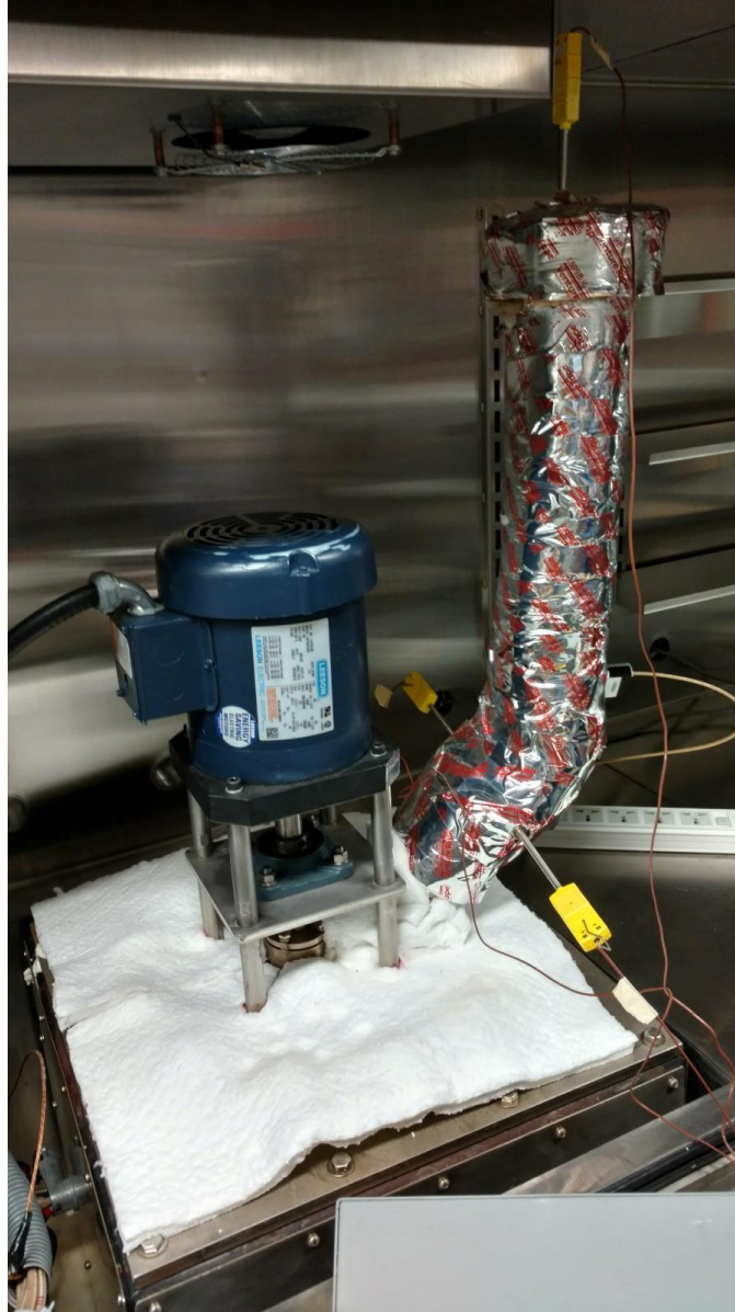
Figure 3-21 Test loop in salt shakedown configuration
